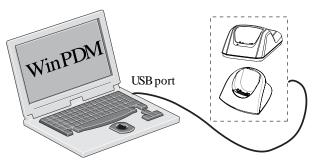
Figure 3: Connection to the computer running WinPDM
